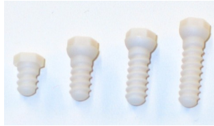
Figure 2: Ceramic screw type from left to right: SA45, SA06, SA08 and SA10
