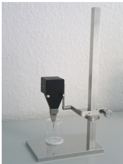
Fig. 3: Labstand for Microdrive
