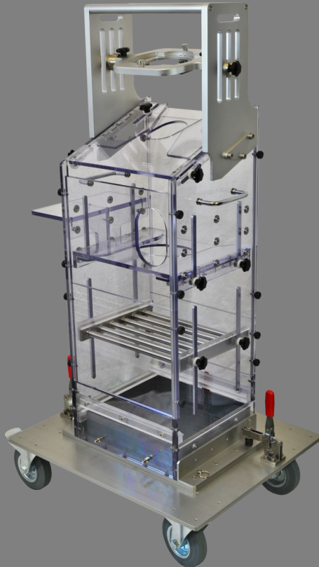
Figure 1: Thomas primate chair with TREC 3-point head holder mounted on a trolley
