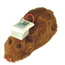
Wireless system for small animals with 4 recording and 1 stimulation channel. Complete system with electrodes, wireless system, battery, and control software.
