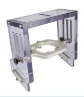
Precision Positioning System (PPS): complete primate stereotaxic instrument with table, frame, curved guided rail, primate chair with trolley, 3 point head holder, reward unit and xyz manipulator for microdrive mounting.
