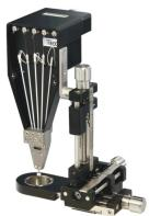
The **Eckhorn Matrix** is available in a 7, 16 motor version for up to 112 signal channels. This drive is mounted to a stereotaxic instrument. The max. electrode travel is 40mm.
