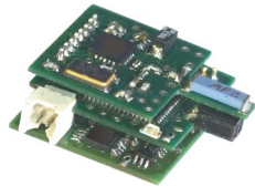
Figure 1: Thomas Dual Stimulator (TDS) without plastic cabinet and accumulator
