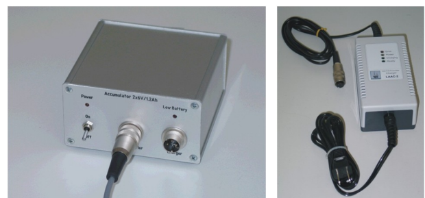
Fig. 2: Accumulator (left) and charger (right) for the Differential PreAmplifier DPA-4
