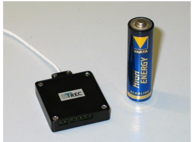
Fig. 1: Differential PreAmplifier DPA-4 in comparison to the size of a standard AA-size battery
