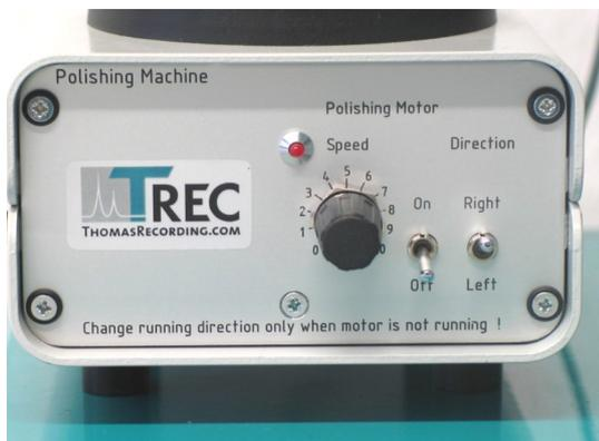
Figure 2: Electrode polishing Machine (EPM-3) control unit front panel
