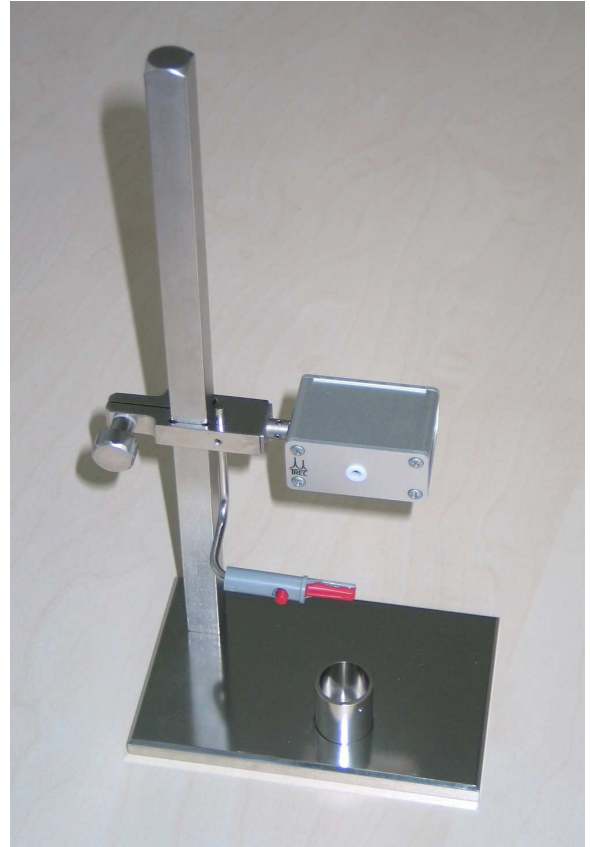
Fig. 3: Laboratory stand with electrode impedance tester preamplifier, electrode holder and beaker for saline solution
