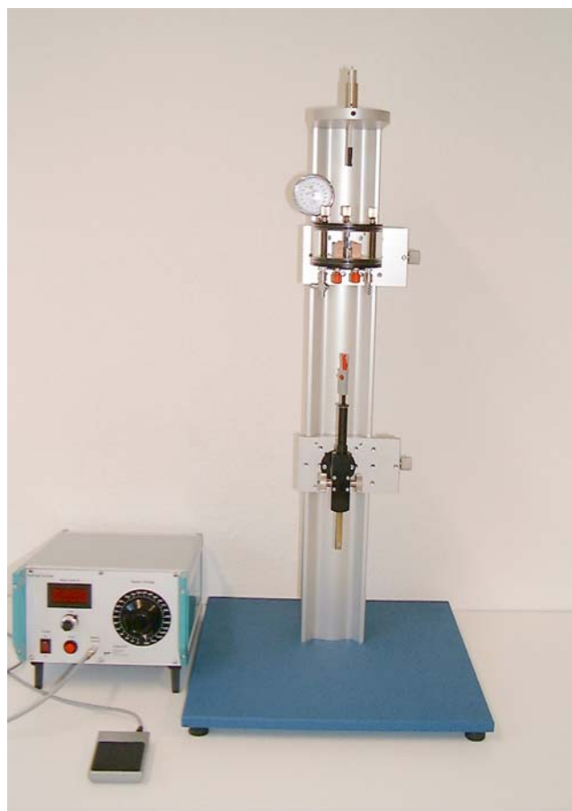
Figure 1: Electrode tip puller ETP-ST (standard version)
