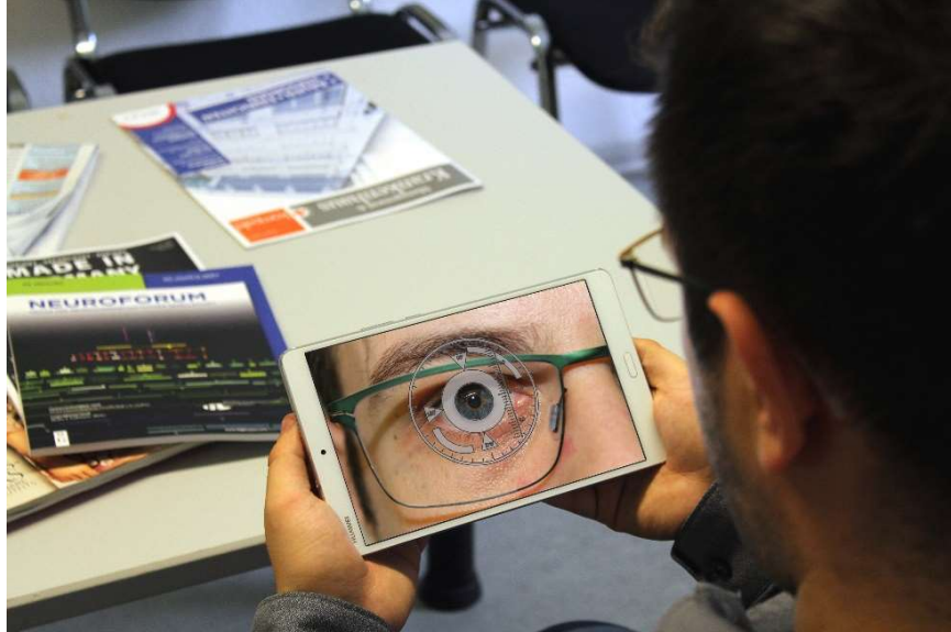
Figure 1: A subject performs an eye movement measurement in the waiting room using a tablet computer
