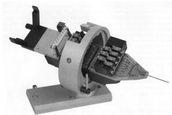
Figure 2: Thomas Microdrive type "Reitboeck Matrix" used by V. B. Mountcastle to place up to 7 fiber microelectrodes in the cortex of non-human primates.
